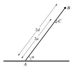
A uniform rod AB has mass m and length 2d. The rod rests in equilibrium on a smooth peg C, with the end A resting on a rough horizontal plane. The distance AC is 2a and the angle between AB and the horizontal is  $\alpha$ , where  $\cos \alpha = \frac{3}{5}$ . A particle of mass  $\frac{1}{2}m$  is attached to the rod at B (see diagram). Find the normal reaction at A and deduce that  $d < \frac{25}{6}a$ .
